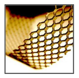
TELPRO Mesh Anodes are manufactured using a titanium expanded mesh substrate, which meets ASTM B265 Grade 1 or Grade 2, which has been coated with TELPRO Mixed Metal Oxide coating.
