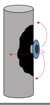
DISC ANODES CAN BE INSTALLED WITH A LOW PROFILE, PREVENTING DAMAGE FROM PASSING SHIPS / CRAFT.
