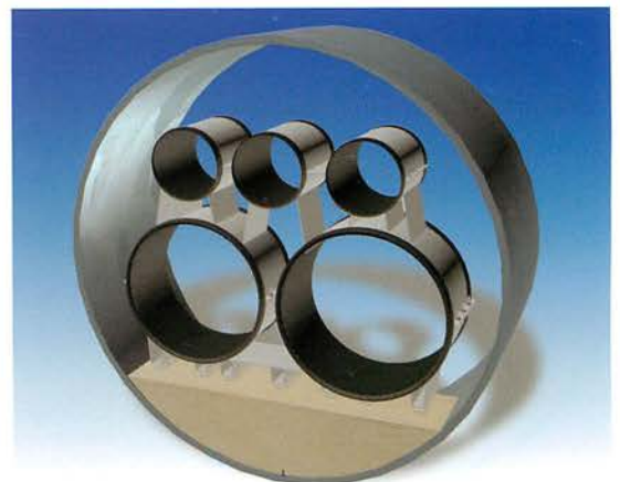
Tunnel Liner Plate Construction with Grout Invert.
