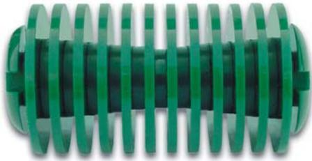
The key to the system is in the design of the process displacement pig, which with its multiple discs, virtually eliminates bypass. The pig is capable of spanning full-branch tees, negotiating full-port valves, and 1.5-diameter bends. The PDP can be manufactured to any diameter, length, and configuration as well as from various compounds to be compatible with different products or applications.
